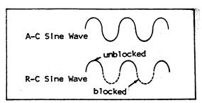
FIGURE 1 - THE RECTIFIED SINE WAVE
